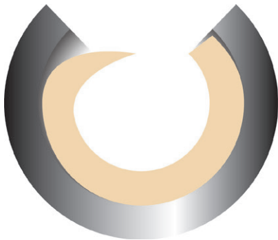
Self-lubricating with teflon liner
