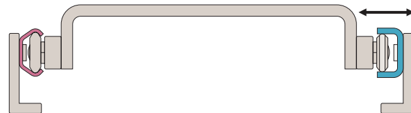
T and U rail allows for misalignment
