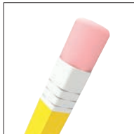
35 durometer: Pencil rubber top
