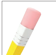
35 durometer: Pencil rubber top
